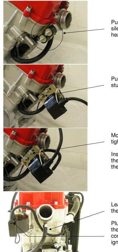
Put the ignition coil onto the two silent blocks on the cylinder head.
