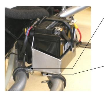
Fix the battery box with the first tube clamp onto the frame.
