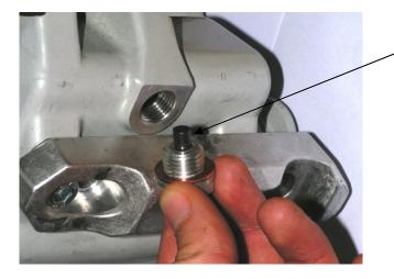
Remove the oil drain plug and clean the magnet on the bolt's end. In case you observe excessive
