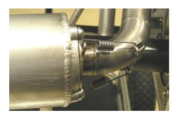
Install the exhaust silencer on a commercially available exhaust bracket (not included in the scope of supply).
