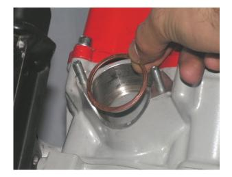
Put the primary tube gasket into the primary tube port.
