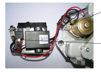
Connect the plus and the minus cable on the battery with the provided slot nuts and bolts.
