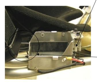
Remove the battery and the rubber floor.
