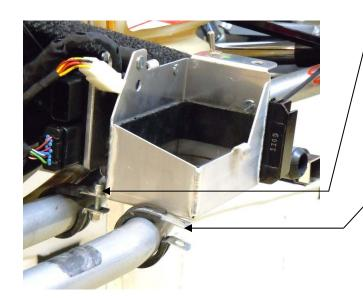
Fix the battery box with the first tube clamp onto the frame.
