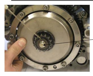
Push the clutch drum backwards and apply chain spray between transmission sprocket and thrust washer.
