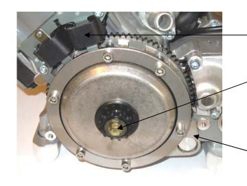
Dismantle the generator stator
