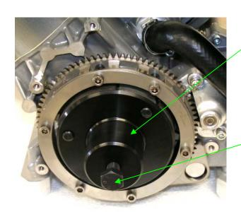
Screw in the clutch puller into the clutch mount by hand as far as possible.
