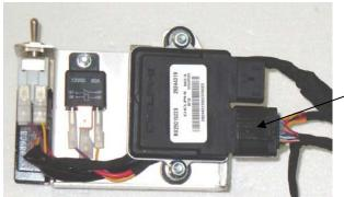
Connect the engine wiring harness to the control unit on the battery box.
