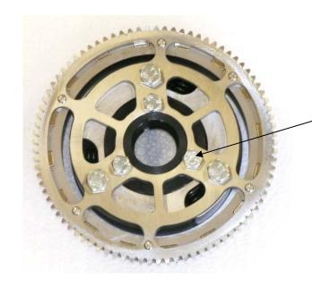
Remove all bolts on the back of the starter sprocket.
