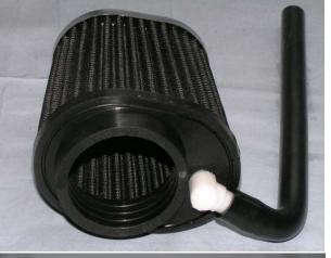
Pull the crankcase ventilation hose onto the ventilation tube and push the tube into the corresponding hole on the air filter.
