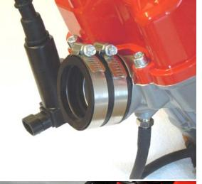
Put the two hose clamps onto the carburetor rubber and push the rubber onto the intake port.
