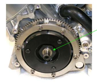
Loosen the clutch mount nut.
