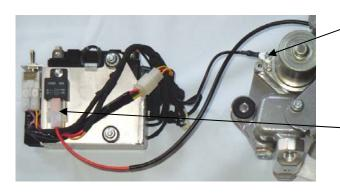
Connect the engine ground cable (black) to the engine.
