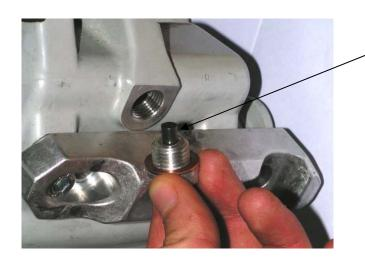
Remove the oil drain plug and clean the magnet on the bolt's end.
