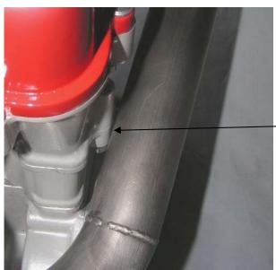
Position the primary tube in that way to leave a gap of 1mm.
