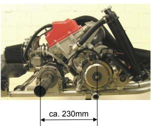
Now install the engine onto the go-kart.
