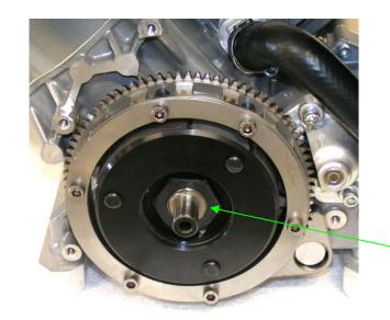
Lock the clutch with the special tool "BATMAN"
