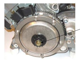
Install the clutch drum and the transmission sprocket bearing. Mount the "BATMAN"-tool.
