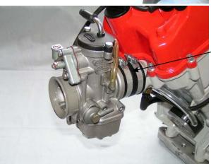
Put the carburetor into the carburetor rubber and tighten both hose clamps.
