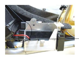
Remove the battery and the rubber floor.
