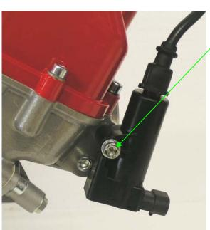
Mount the ignition coil as shown on the cylinder head.
