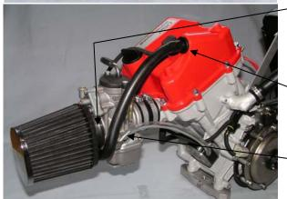
Install the air filter onto the carburetor and tighten the hose clamp.
