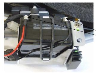
Connect the plus and the minus cable on the battery with the provided slot nuts and bolts.
