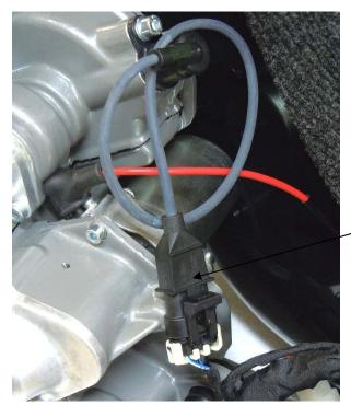
Connect the engine wiring harness with the crank shaft trigger sensor.
