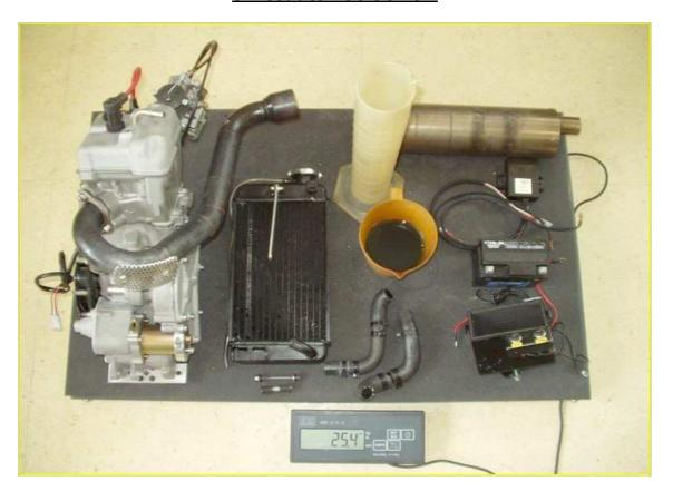
While the 2 stroke base engine weighs only about 12 kg, the whole system brings another 14 kg to a total of around 26 kg of the whole system weight onto the scale.
