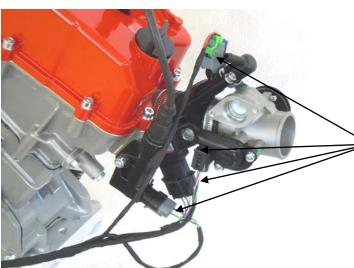
Connect the injector nozzle, throttle position sensor, MAP sensor and the ignition coil.
