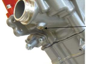
Close the hole with the screw plug Use Loctite 577
