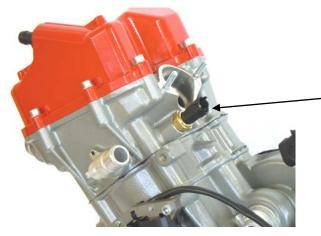
Install the water temperature sensor.
