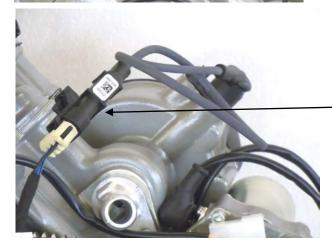
Connect the crank trigger sensor.
