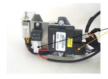
Install the reprogrammed or exchanged EFI ECU.
