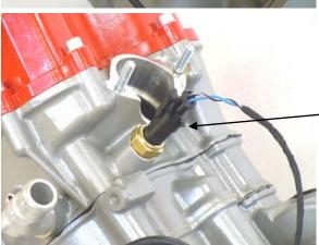
Connect the water temperature sensor.
