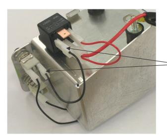
Remove the black cable from the start switch to the starter relay.
