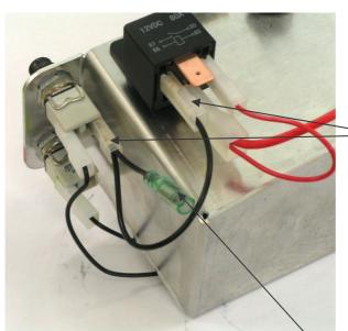
Connect the delivered new cable with the start switch and the starter relay.
