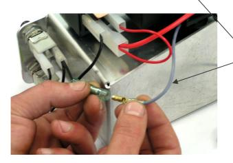
Install the new control unit and connect the grey cable of the control unit with the free plug of the new cable.
