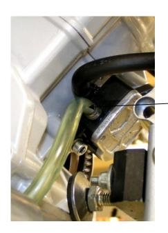
Lead the gas line to the fuel pump and connect it to the free position on the fuel pump.
