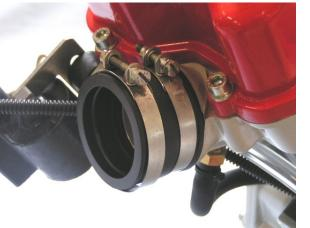
Put the two hose clamps onto the carburetor rubber and push the rubber onto the intake port.
