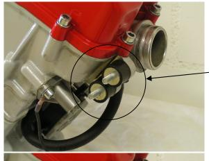
Put the ignition coil onto the two silent blocks on the cylinder head.
