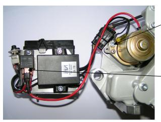
Connect the engine ground cable (black) to the engine.
