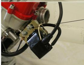
Mount both flange nuts and tighten the nuts with 10Nm.
