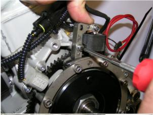
Slide the bent feeler gauge of 1.2mm between primary coil and magneto.
