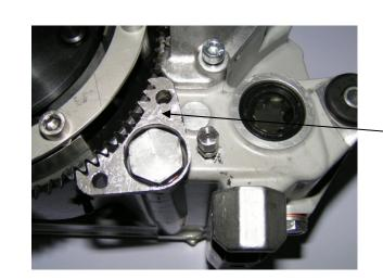
Lock the clutch with the special tool "BATMAN".
