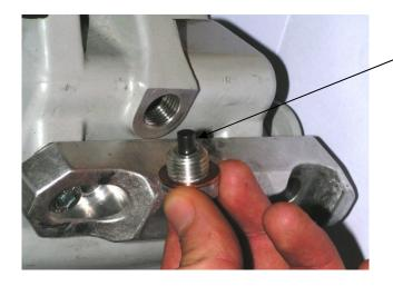
Remove the oil drain plug and clean the magnet on the bolt's end.
