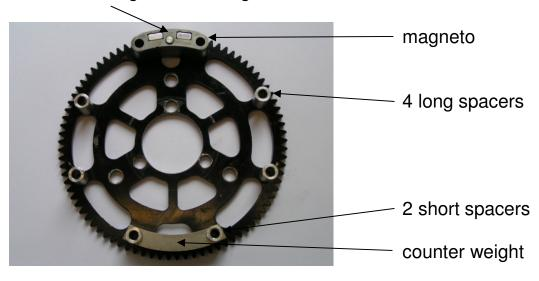
Put the supporting ring with the 9 holes onto the sprocket and tighten the unit with 8 stainless steel M6 bolts by applying a torque of 10Nm.
