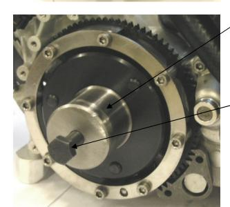
Screw in the clutch puller into the clutch mount by hand as far as possible.
