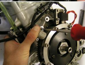
Remove the "BATMAN"-tool and turn the crankshaft till the counter weight and the pick-up are in line.
