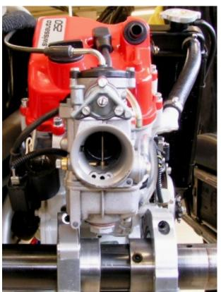
Install the inner wire of the throttle cable on the carburetor and lead the wire with the cable sleeve along the seat.
