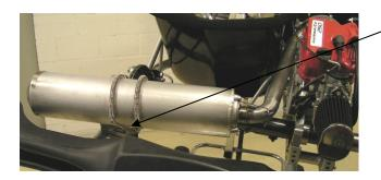
Install the exhaust silencer on a commercially available exhaust bracket (not included in the scope of supply).
