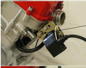
Put the ground cable onto the stud of the lower silent block.
