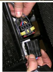
Connect the engine wiring harness to the control unit on the battery box.
