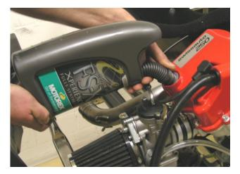
Fill in 0.4l 0W30 motor oil from "Motorex" into the engine.
