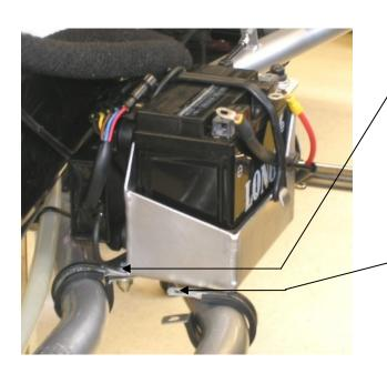
Fix the battery box with the first tube clamp onto the frame.
