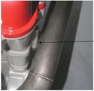
Position the primary tube in that way to leave a gap of 1mm.
