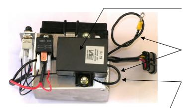
Install the control unit onto the two silent blocks and tighten both flange nuts M6.
