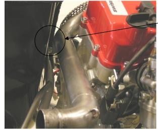
The distance between primary tube and driver seat should result in min. 2cm.
