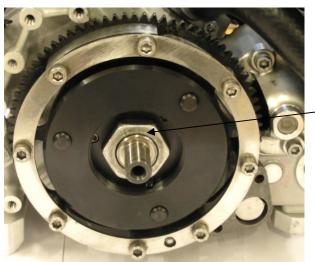
Loosen the clutch mount nut.
