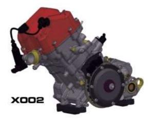
The VT1 – swissauto250 spare engine is thought as a quick replacement engine. It comes <u>without</u> exhaust system, carburetor/throttle body, air-filter, radiator, battery box, and ECU. It does have a mounted clutch, fuel-pump, charge coil, ignition coil, pick-up sensor and the engine mounts. It definitely is the cheapest way to have a second swissauto250 race engine.
